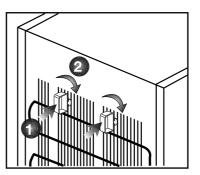
order to allow the air circulation. (The illustrated figure is only an example and does not match exactly with your product.)
